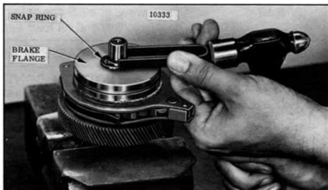
Figure 5-6. Remove Snap Ring From Load Brake Shaft.
